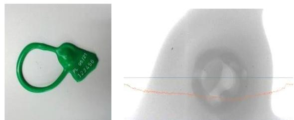
Fig. 10 Photo of the damaged PL 95 type seal and a view into the structure of the security component after thermal deformation (185°C)
