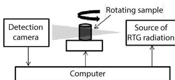
Fig. 1 The diagram of x-ray microtomography function
