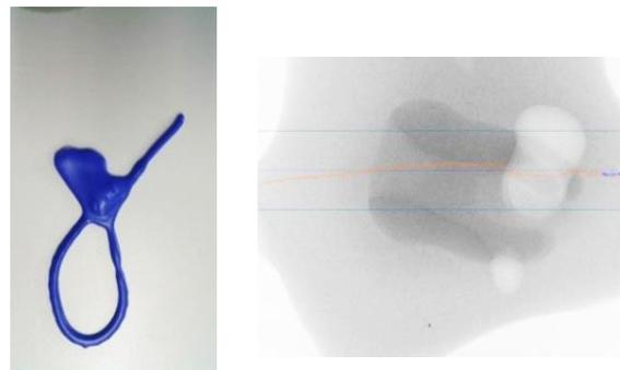
Fig. 9 Photo of a badly damaged seal of the PL 91 type and a view provided by the tomograph into the structure of the security component damaged by thermal deformation (185°C)
