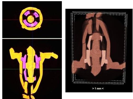
Fig. 8 A cut through seal of the PL type deformed by heat (120°C) and a 3D model of the destroyed seal
