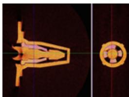
Fig. 14 Visualization of the PL 95 type security seal after chemical damage cause by Polyoxymethylen
