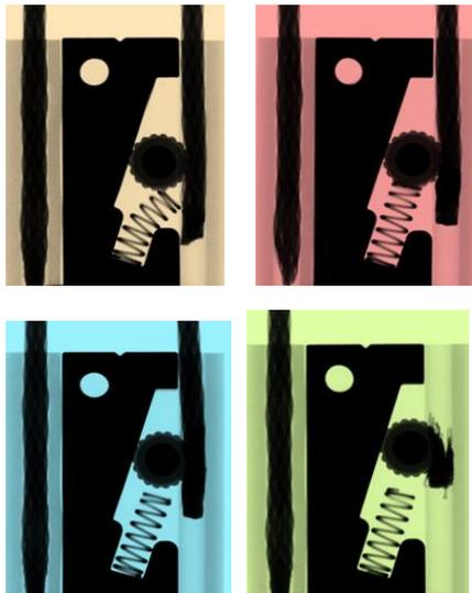
Fig. 12 Visualization of the tensile deformation of the metal security components (strained by 1, 2, 3 and 4.4 kN – from left to right)
