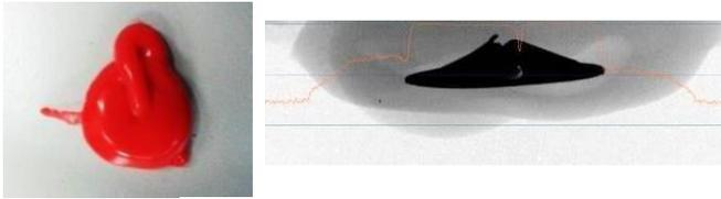
Fig. 11 Photo of the damaged ES type seal and a view provided by the tomograph onto the structure of the security component after thermal deformation (185°C)
