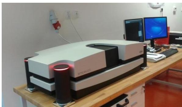
Fig. 2 Microtomographic device SkyScan 1272 including the workstation
