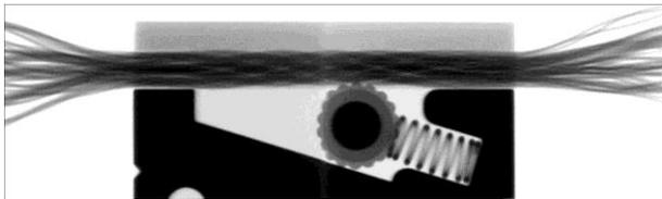
Fig. 6 Visualization of the metal cable seals
