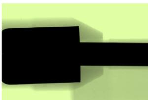
Fig. 7 Image provided by the scanner – metal cable seal
